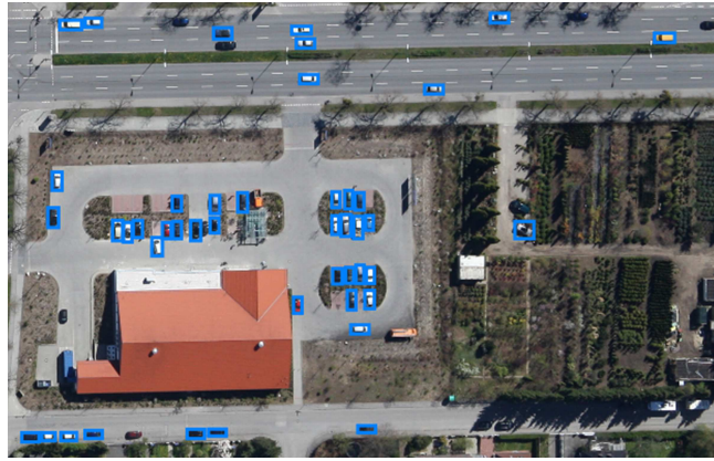
Fig. 3: Vehicle detection result using ShuffleDet on the 3K-DLR-Munich dataset.
