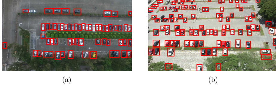
Fig. 2: Sample vehicle detection results using ShuffleDet on the CARPK(a) dataset and the PUCPR+ dataset(b). mostly due to our tuned scales and aspect ratios. This effect can also be observed between the original implementation of Faster-RCNN with and without small RPNs.
