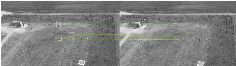
(b) Example result for object center tracking with sparse optical flow on our in-house captured video.
