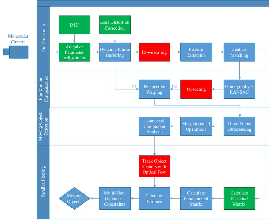
Fig. 1: Our proposed moving object detection pipeline. Red boxes represent the steps we build on other baselines. Green boxes represent steps that can be applied where IMU and camera calibration parameters are available.  $F_o$  represents the frame in original resolution and  $H_u$  represents upscaled homography.
