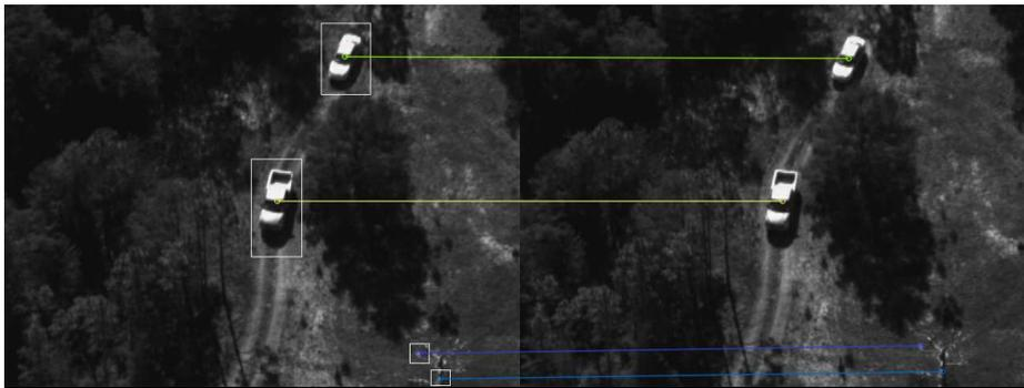
(b) Example result for object center tracking with sparse optical flow on EgTest05.
