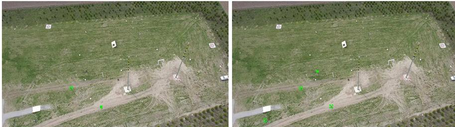
(c) Image (b) processed with a static buffer size parameter used in subfigure (a). (d) Image (b) processed with dynamically adjusted buffer size.
