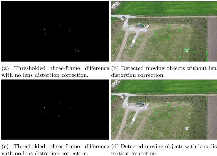
Fig. 7: The effect of lens distortion correction. Note that although the effects of lens correction on input images may be almost imperceptible, it gives rise to many pixel level errors.
