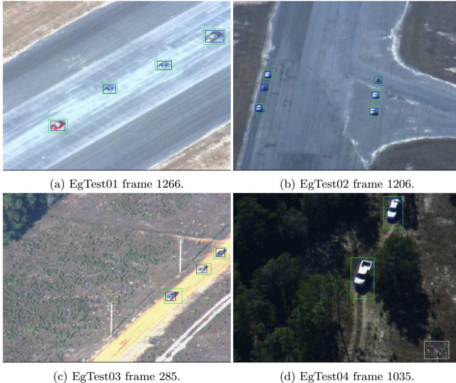
Fig. 6: Detection results on 4 sequences of VIVID dataset. Green boxes are detection results, blue boxes are ground truth data that are taken from LAMOD dataset, grey boxes are candidate objects that are filtered by our parallax filtering algorithm.
