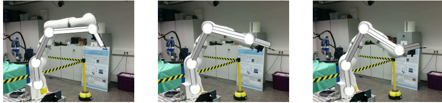
Fig. 7. Reconstruction of the sword play sequence of the CMU database. The kinematic chain is extended such that the hands are rigidly connected.
