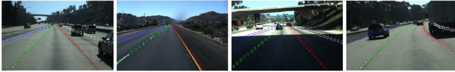
Fig. 1. Example of multilane detection and classification by our network, where the output is in the form of lane boundary image coordinates represented by small color circles (best viewed on computer screen when zoomed in). Classified leftside , leftego , rightego and rightside lane boundaries are represented by blue, green, red and white colors respectively (best seen in color)
