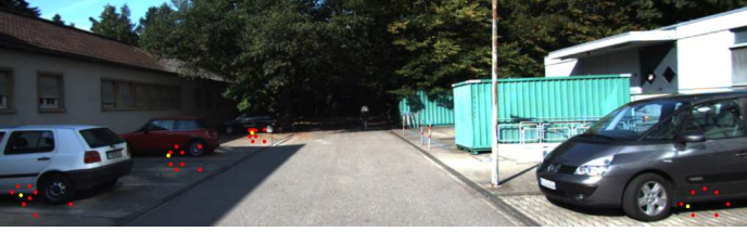
Fig. 2: The red circle shows the center of positive anchors selected by our approach and the yellow circle shows the projection of the center of the ground truth 3D bounding box. In comparison to IOU(Intersection Over Union) based anchor labeling approach, we label very few anchors as positive. Also depending upon the size of the anchor, IOU of the positive anchor with the object can be less than 0.5.
