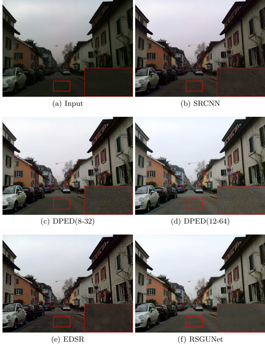
Fig. 4. Enhanced images by different methods using (a) as input. m - n means the model has m convolution layers with each layer having n channels.
