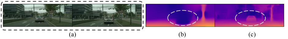
Fig. 3: Moving object in the scene (a) causes large depth value confusion for framework trained with monocular videos, as shown in (b). This issue can be resolved by incorporating stereo training samples into the framework (c).
