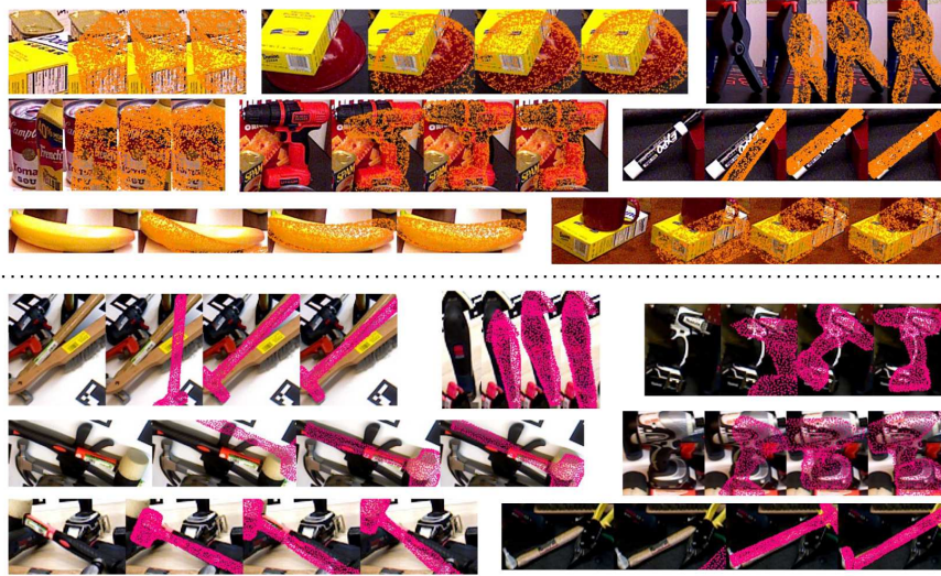
Fig. 4: Illustration of pose estimation results by MCN on YCB-Video (upper) and JHUScene-50 (bottom). The projected object mesh points that are transformed by pose estimates are highlighted by orange (YCB-Video) and pink (JHUScene-50). From left to right of each data, we show original ROI, MCN estimates on RGB, MCN estimates on RGB-D and MV5-MCN estimates on RGB-D.
