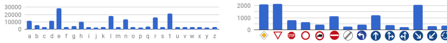
Fig. 3. Number of points in each class of EMNIST (left) and GTSRB (right) databases.
