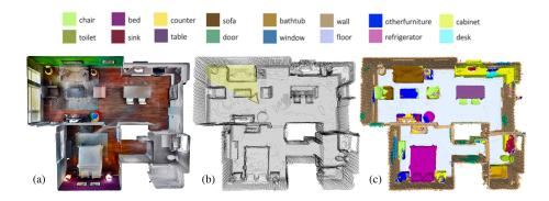
Fig. 1: Example result of our FCPN on semantic voxel labeling and captioning on an Tango 3D reconstruction / point cloud: (a) 3D reconstruction (not used), (b) Input point cloud (c) Output semantic voxel prediction. A possible caption for the camera pose in (b) is "There is a place to sit in front of you"
