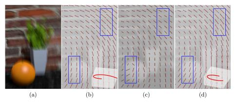
Fig. 4: Example of camera motion initialization on a synthetic light field. (a) Blurred input light field. (b) Ground truth motion flow. (c) Sun et al. [30] (EPE = 3.05), (d) Proposed initial motion (EPE = 0.95). In (b) and (d), the linear blur kernels are approximated only using the end points of camera motion for the visualization.
