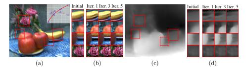
Fig. 3: Example of the iterative joint estimation. The proposed method converges in small number of iteration. (a) $\sim$ (b) Input blurred image and deblurring results by iteration. (c) $\sim$ (d) Initial blurred depth map and depth estimation results by iteration.
