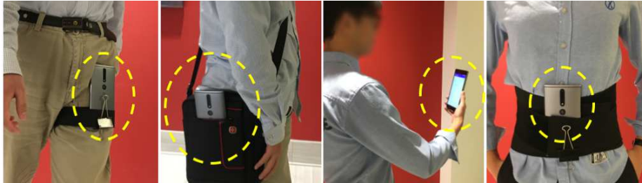
Fig. 2. We place a Tango phone in four popular configurations to collect training data. The ground truth motions come from Visual Inertial Odometry, and we have carefully designed the placements to make the camera always visible. From left to right: 1) in a leg pocket, 2) in a bag, 3) held by a hand, or 4) on a body (e.g., for officers).
