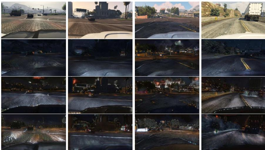
Fig. 3: **GTA** day-to-night transformation results - GANs trained with **GTA**: First row: GTA daytime testing images; Second row: outputs of CycleGAN; 3rd row: outputs of UNIT; 4th row: outputs of AugGAN.
