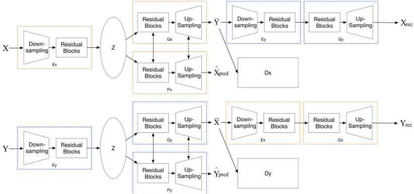
Fig. 1: Overall structure of the proposed image-to-image translation network.  $X$ ,  $Y$ : image domain  $X$  and  $Y$ ;  $Z$ : feature domain;  $\hat{X}_{pred}$ ,  $\hat{Y}_{pred}$ : predicted segmentation masks;  $\bar{X}$ ,  $\bar{Y}$ : translated results; dotted line implicates soft-sharing, solid line implicates hard-sharing.
