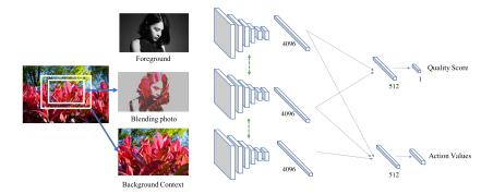
Fig. 5. Network structure of the proposed policy network. We extend the quality network with an additional background context input and action values output. The designed structure enables the agent to jointly predict the quality value as well as search action values, reducing the time complexity during the process of parameter search.
