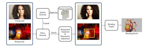
**Fig. 2.** Overview of the automatic blending framework. The inputs of our method are two photos: foreground and background. We first train a quality network to evaluate the aesthetics quality of blending photos with human preference annotation on random blending photos. Then a deep reinforcement learning based agent is trained to optimize the parameter for the background alignment and photometric adjustment. Using the predicted parameters, the blending engine renders the final blending photo.
