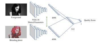
Fig. 3. Network structure of the proposed quality network. The quality network consists of two of VGG16 networks that share the same parameters. The quality network takes the original foreground photo and the blending results as input and outputs a numeric score that indicates the aesthetic quality of the blending result.
