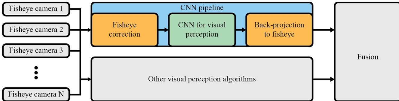
Figure 1: Typical processing block diagram for a surround view (SV) camera system. The convolutional neural network (CNN) algorithms for visual perception often have two additional steps (i.e., fisheye correction and back-projection to fisheye space). These steps are undesirable as they may become a bottleneck in achieving real-time performance.
