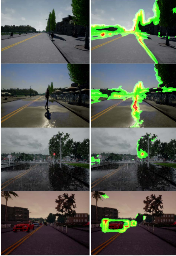
Figure 5: VisualBackprop (right) for ego trajectory prediction and corresponding image (left), best viewed in color. The heatmap overlay represents area of activation (green is low and red is high). From top to bottom: ego car too close to the sidewalk, pedestrian crossing, before stopping at red light, dense traffic
