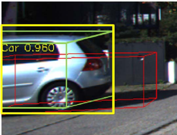
Figure 5. Truncated detection box example. Yellow line is the 2D detection box, and x_{\min} is clipped to zero. Green line illustrates the reconstructed 3D box using the iterative method. Red line is the reconstructed 3D box obtained from all 2D box parameters. If we use the clipped value of x_{\min} = 0 , the ray vector is ((0.5x_{\max} - c_x)/f_x, 1) .
