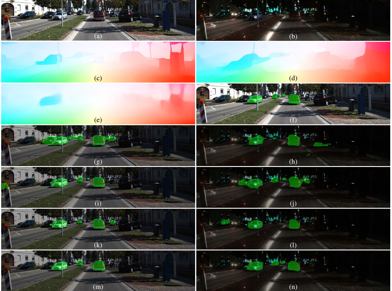
Figure 5: Qualitative comparison of our algorithm on KITTI and Dark-KITTI datasets. First column shows inputs and results on KITTI while second shows results on Dark-KITTI. (a),(b) show the input RGB images. (c),(d) show rgbFlow. (e) shows lidarFlow. (f) shows Ground Truth. (g),(h) show output using RGB-only. (i),(j) show output of (RGB + rgbFlow). (k),(l) show output of (RGB + lidarFlow). (m),(n) show output of (RGB + rgbFlow + lidarFlow).
