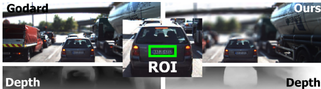
Figure 9: Experiments on real data. The region of interest is set with 2D tracking onto the number plate (middle) and the corresponding depth value is recovered. The left illustrates refocusing using a depth map generated by [14] while we show on the right the result of our sequential refocusing pipeline, together with the underlying disparity map.
