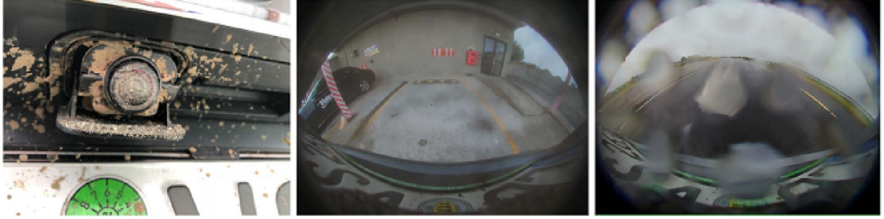
Figure 1: From left to right: a) soiled camera lens mounted to the car body; b) the image quality of the soiled camera from the previous image; c) an example of image soiled by a heavy rain.
