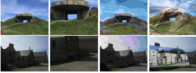
Figure 8: Near-duplicate samples from the INRIA CopyDays dataset. From left to right the image types: original image, crop, JPEG compression, strongly attacked. The strongly attacked types include print and scan, blur, paint. These distorted versions are regarded as near-duplicate for each other.
