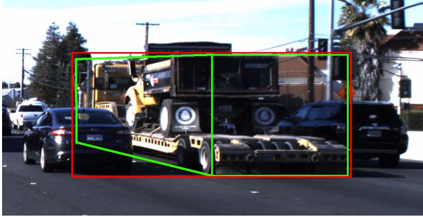
Figure 5. The difference in accuracy between 2D and 3D annotations. The 2D axis-aligned bounding box clearly includes parts of a neighboring lane.
