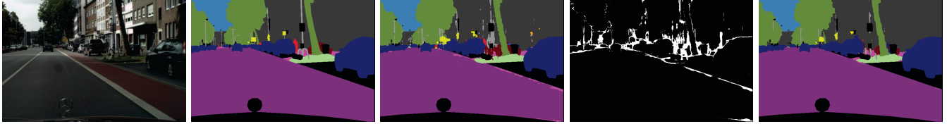
Figure 1: From left to right: sample image from Cityscapes [6], corresponding ground-truth image, predictions from U-Net trained with cross-entropy loss, betting map from the gambler network, predictions from the gambling adversarial nets. Notice e.g. spotted and resolved artefact in predictions from the cross-entropy trained U-Net in bottom right and right side of the road. Best visible zoomed-in on a screen. Black area on the labels and predictions represents the void-class, that is excluded in the evaluation [6]
