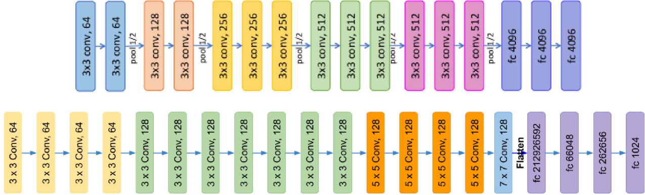
Figure 2. The VGG16 network (top) and our modified variant (bottom) used for the recognition task.
