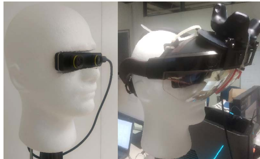
Figure 1. The mannequin head used to perform the calibration.
