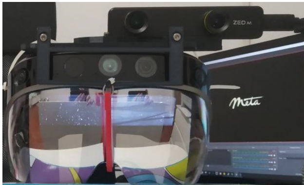
Figure 5. Calibration of the ZED camera with the Meta2 camera, needed to obtain the transformation matrix {}^Z_C\mathbf{T} that defines their relative pose.
