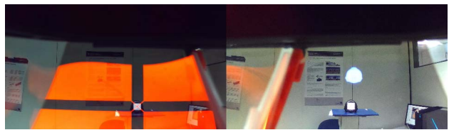
Figure 6. The view from inside the HMD during the alignment task while calibrating the left eye. On the right lens, the bright hologram floating several decimeters above the tracker shows the current uncalibrated reprojection.
