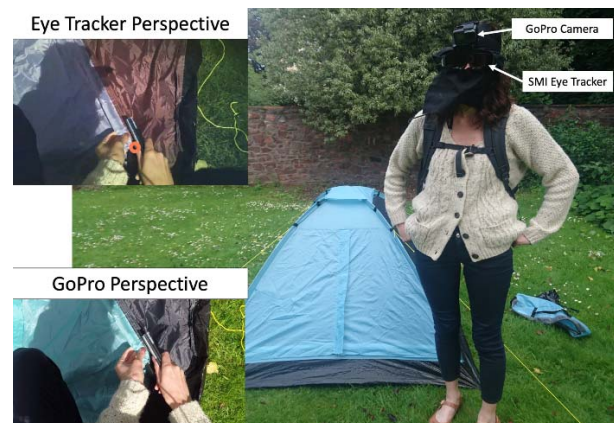
Figure 1. Participant standing next to a completed tent, wearing the GoPro and SMI eye tracker. To avoid the sun's infrared interference, the eye tracker was outfitted with protective lenses and black cloth. (Top Left) Egocentric perspective from the SMI camera, the orange circle represents the participant's point of gaze. (Bottom Left) Egocentric perspective from the GoPro camera.
