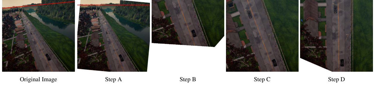
Figure 3: Step-by-step transformations of the first image to obtain the desired bird's eye view. The different sub-figures correspond to images obtained after performing the steps described in section 3 for predicting the homography matrix.
