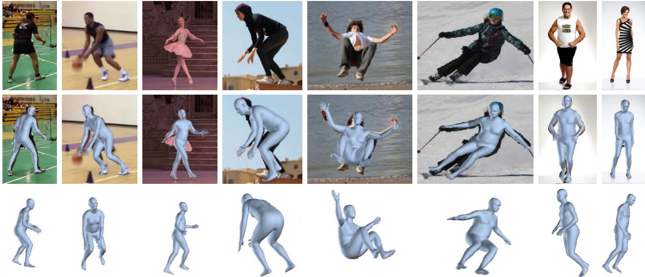
Figure 1. Results of our human shape reconstruction on challenging examples. The first row shows the input images, the second row shows the reconstruction results, and the third row show the reconstructed body at novel views.
