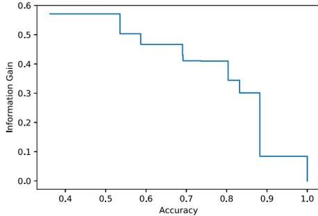
(c) Accuracy vs. information gain using ResNet as off-the-shelf classifier on ILSVRC1K
