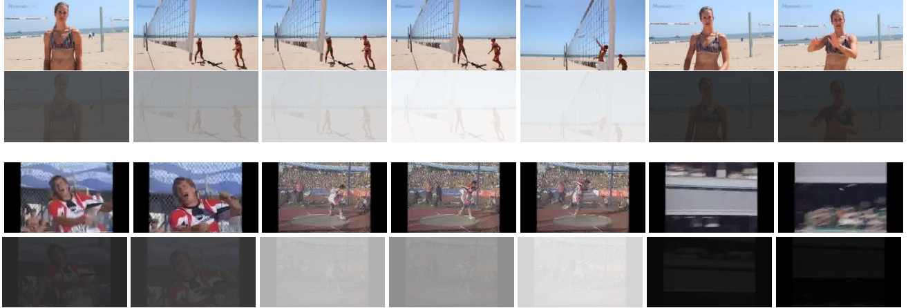
Figure 6. Examples of temporal attention from THUMOS14. The upper two rows show original images of the Volleyball action, and the corresponding images overlaid with temporal attention weights. The lower two rows show the Throw Discus action. Our temporal attention module can automatically highlight important frames and avoid irrelevant frames corresponding to non-action poses or background.
