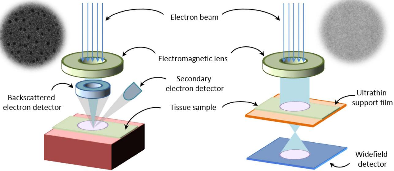
Figure 1: Schematic of SEM (left) and TEM (right) image acquisition workflows accompanied by examples of associated artifacts (noise pattern).
