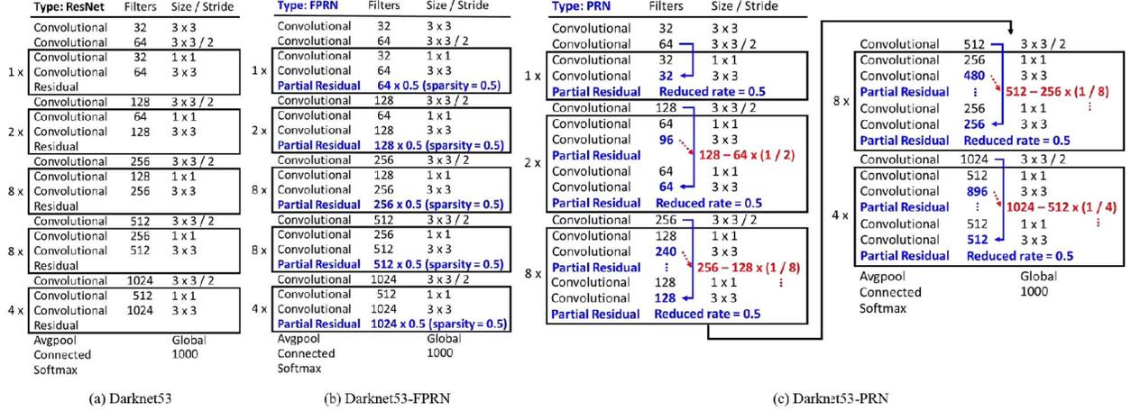
Figure 7. Architectures of Darknet53, Darknet53-FPRN, and Darknet53-PRN.
