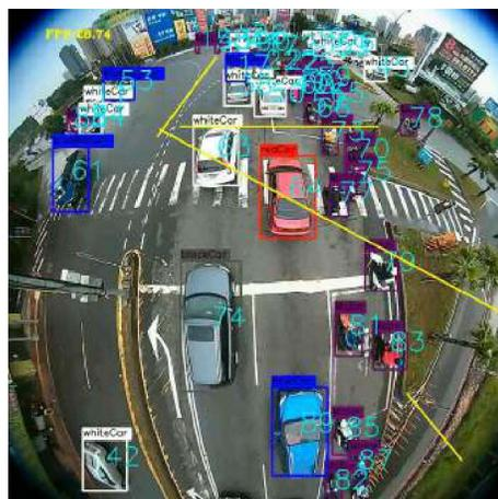
Figure 13. Fisheye lens-based traffic analysis system.
