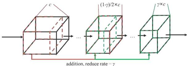
Figure 3. Characteristic 2: Set reduce rate  $= \gamma$ , the number of channels linearly decremented to  $\gamma \times c$ , partial residual connection operates on feature maps with different channel numbers in the same stage.
