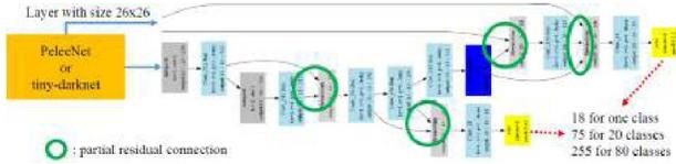
Figure 8. Architecture of tiny PRN head.
