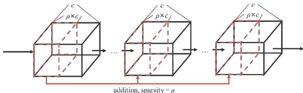
Figure 2. Characteristic 1: maintain the topology of ResNet, change offset, use sparsity  $= \rho$  as the basis for partial residual connection.
