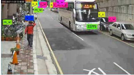
Figure 15. Road licence plate recognition system.
