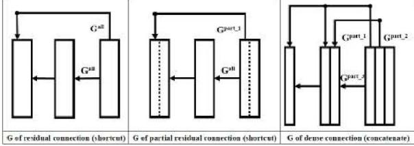
Figure 6. Shortcut connection and concatenate have different gradient propagation sources.
