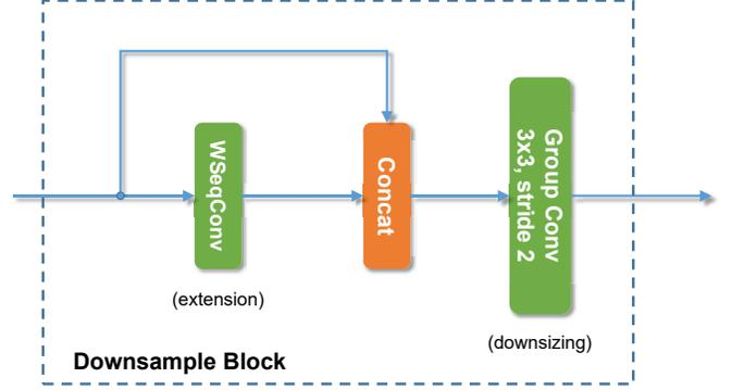
Figure 3. The topology of a down-sampling block, the extension layer and downsizing layer are, respectively, implemented by a WSeqConv layer and a grouped Conv layer of stride 2.
