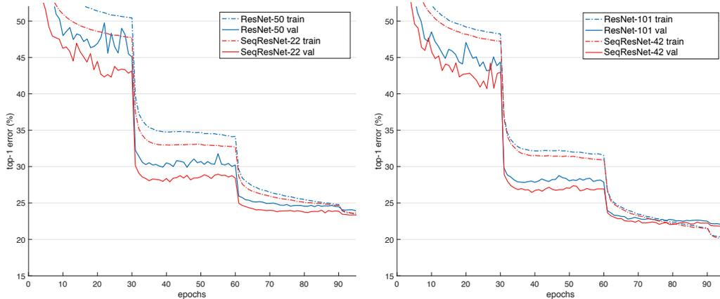
Figure 4. Training curves of SeqResNet-B22/ResNet-50 (left) and SeqResNet-B42/ResNet-101 (right) on ImageNet.
