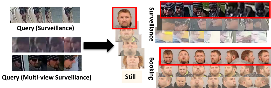
Figure 2: Surveillance video protocols in IJB-S dataset [21]. The queries are on the left and the galleries are on the right of the arrow. In each protocol, the query is either one surveillance video or multiple videos of the same person, which needs to be compared with every item in one of the three galleries types (still images, surveillance videos, and booking photos). The red boxes are used to highlight the ground truth identity. Since faces are difficult to detect in UAV videos, we only show examples for four of the five protocols.
