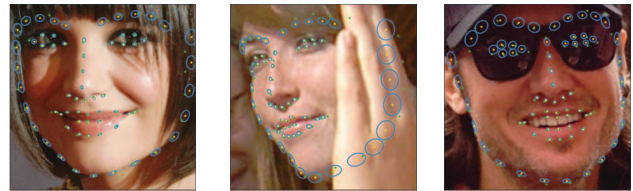
Figure 1: Results of our joint face alignment and uncertainty estimation on three test images. Ground truth (green) and predicted (yellow) landmark locations are shown. The estimated uncertainty of the predicted location of each landmark is shown in blue (Gaussian error ellipse for Mahalanobis distance 1). Landmarks that are occluded (e.g., by the hand in center image) tend to have larger uncertainty.
