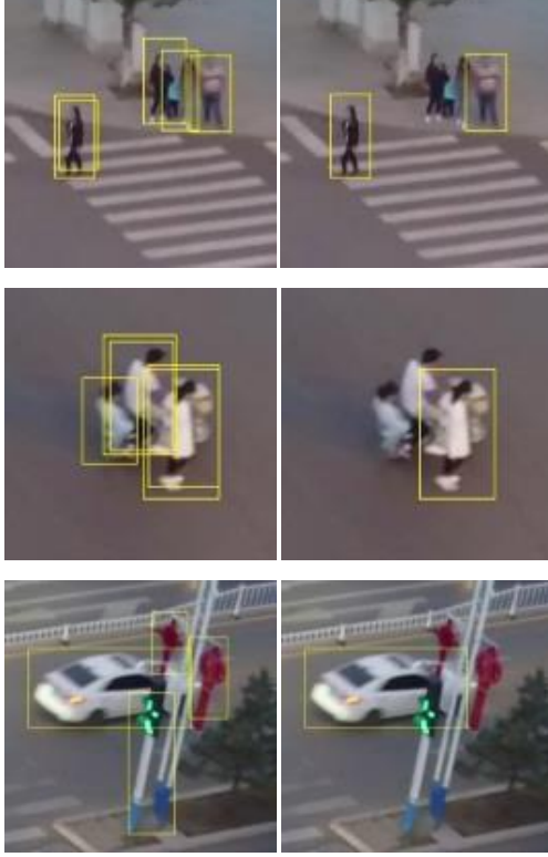
Figure 3. Sample detection filtering outputs using IOU Tracker. Left column: detection results of CenterNet. Right column: refined detection results after filtering.
