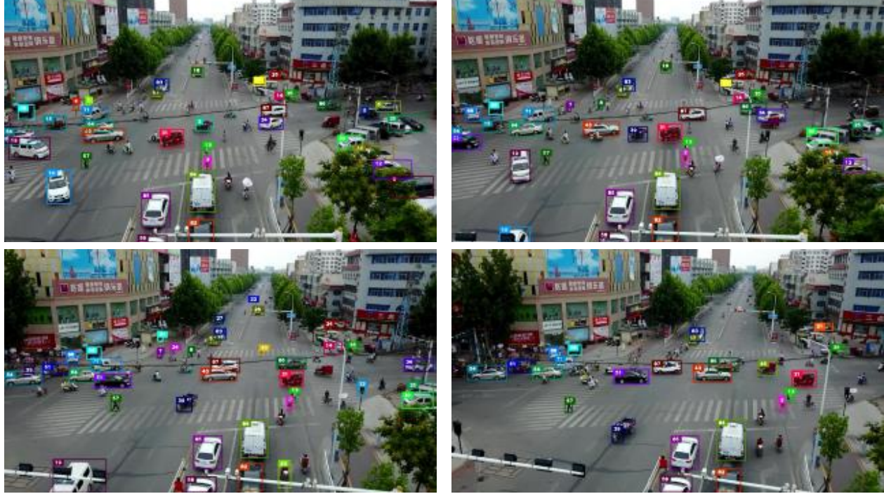
Figure 5. A tracking example of the proposed method. The tracks are identified by the color of bounding boxes.
