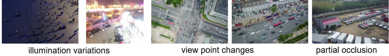
Figure 1. The challenges in the UAV vision. Objects are small and densely distributed with partial occlusion and illumination variations. The viewpoint changed due to the different height of drones and camera directions.
