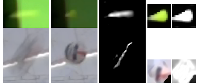
Input I High FPS Blur H F M Figure 7. Deblatting examples. From left to right: the input image, corresponding high-speed camera frame, estimated blur H , estimated appearance F and shape M .
