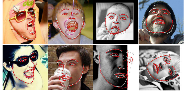
Figure 4: Fittings with the highest error from 300-W test set (first row) and Menpo (second row) (NME 6.5-7%). Red: ground truth. White: our predictions. In most cases, our predictions are more accurate than the ground truth.
