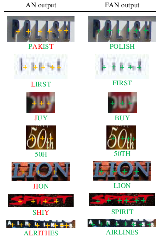
Figure 5. Some real images processed by AN and FAN. The left and right columns are the output results of AN and FAN respectively. The predicted text string for each input image is shown just below the image. The attention centers are marked as ‘+’ of yellow (for AN) and green (for FAN). Green/red characters indicate correctly/incorrectly recognized characters.
