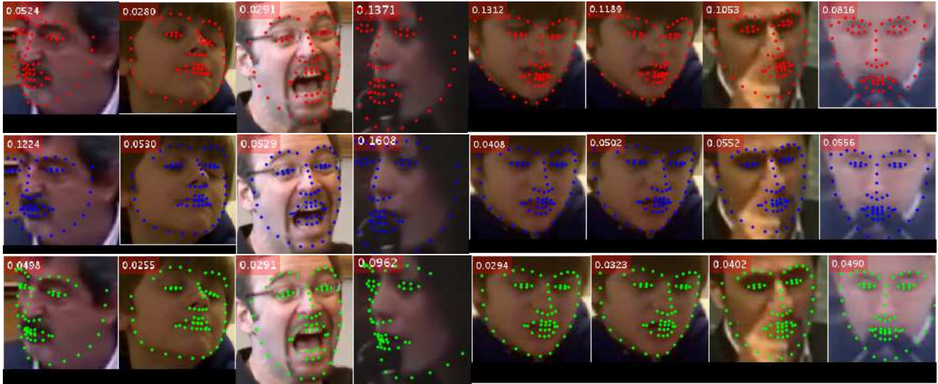
Figure 2. First row (red): Tracking fittings. Second row (blue): Detection fittings. Third row (green): DGCM fittings. The normalized error for each fitting is displayed on the top-left corner. First 4 images (from left to right): Tracker works better than the detector. Last 4 images: Detector works better than the tracker. In all 8 cases, DGCM works better or comparably with the second best performing method.
