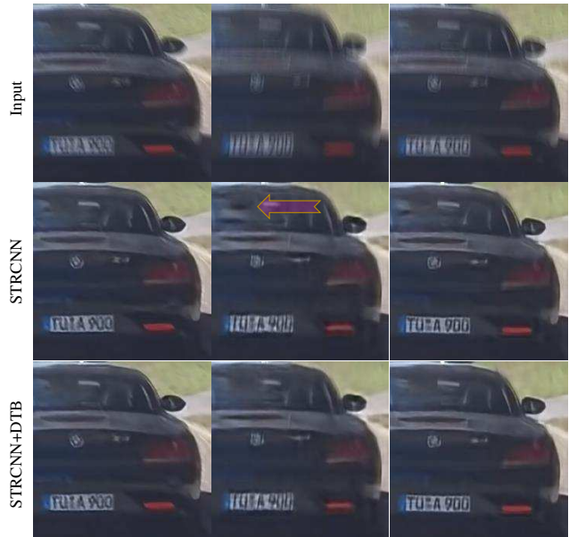
Figure 6: Top to bottom: Consecutive blurry frames, deblurred results by STRCNN and STRCNN+DTB. Notably, the arrow indicates erroneous region by STRCNN model.
