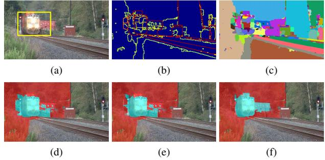
Figure 3. The ASE segmentation of a frame in the “Train0001” sequence: (a) input frame with a bounding box  $b_i^{(t)}$ , (b) UCM, (c) superpixels, (d) preliminary classification, (e) intra-frame refinement, and (f) inter-frame refinement.
