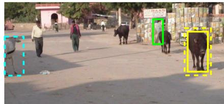
Figure 2. Joint detection and tracking. Dotted and solid rectangles represent detection and tracking boxes, respectively.
