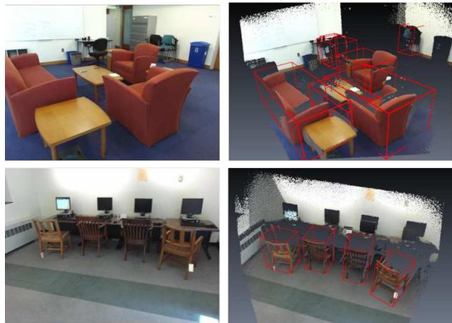
Figure 1. Output of our 2D-driven 3D detection method. Given an RGB image (left) and its corresponding depth image, we place 3D bounding boxes around objects of a known class (right). We make best use of 2D object detection methods to hone in at possible object locations and place 3D bounding boxes.
