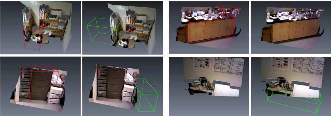
Figure 6. False detections from our proposed technique, including objects that are not detected in 2D, objects that are misplaced using the output of the MLP, and false positives from unseen object classes, but look similar to a class in the training set (counter vs desk, drawer vs dresser).
