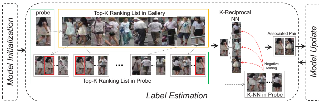
Figure 2. The pipeline of the proposed approach (best viewed in color). After model initialization, several candidates of a given probe are selected and refined via the K-reciprocal nearest neighbor searching and negative mining. Cross-camera tracklets associated with this query are located and used to updated the model. Model updating and sample association stop when no more cross-camera tracklet pairs are generated.
