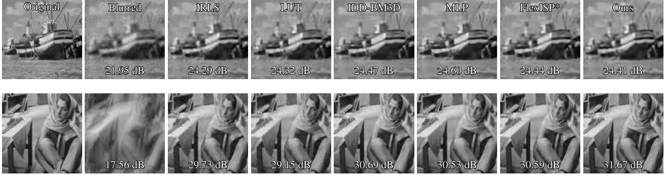
Figure 5: Visual comparison of different deconvolution methods on two out of 11 standard test images. The images Boat and Barbara were each corrupted with Gaussian noise ( \sigma = 0.04 , \sigma = 0.01 ) and a Gaussian blur (experiment a ) as well as a motion blur (experiment e ), respectively. Apart from FlexISP* and our result, all other images are taken from [18].
