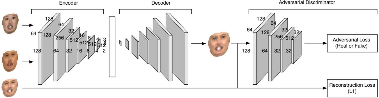
Figure 2. The network architecture. The encoder takes as input the identity texture and the expression texture, and the decoder outputs the dynamic texture. The adversarial discriminator is used during training to judge whether the output texture looks real or not.
