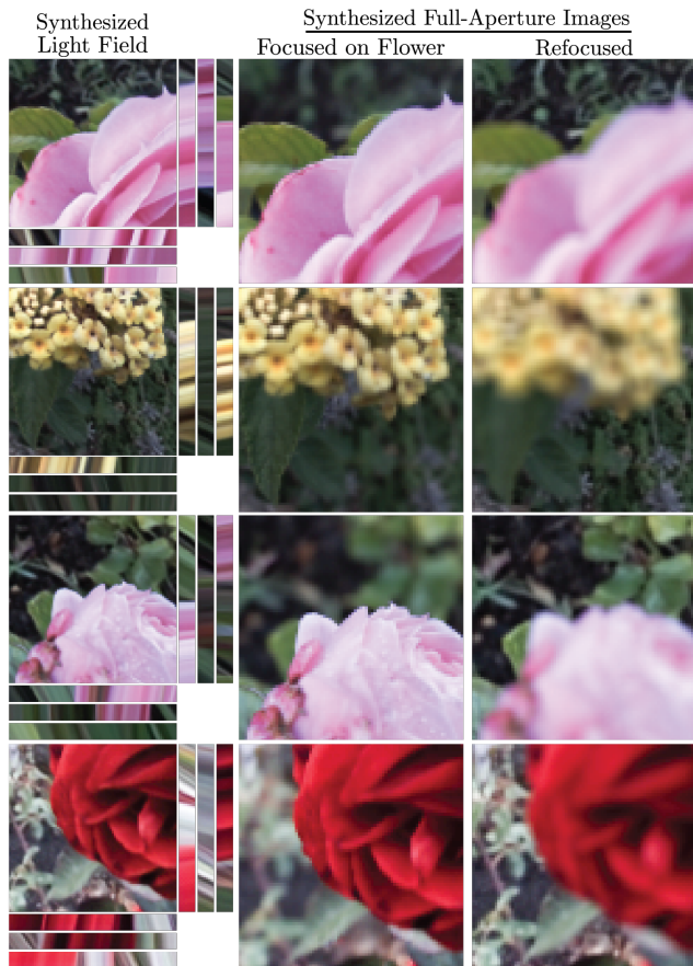
Figure 9. We visualize our synthesized light fields as a corner view crop, along with several epipolar slice crops. The epipolar slices demonstrate that our synthesized light fields contain complex occlusions and relative depths. We additionally demonstrate that our light field generated from a single 2D image can be used for synthetic defocus blur, increasing the aperture from f/28 to f/3.5 . Moreover, we can use our light fields to convincingly refocus the full-aperture image from the flowers to the background.
