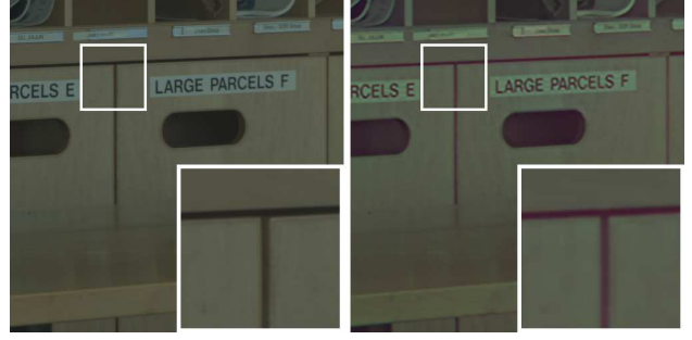
Figure 4: Left: ground truth image; right: recovered image using 0-order CCT initialization. Notice that in the zoom-in insets the black lines have turn red.
