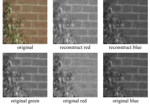
Figure 3: Results of our similarity model tested on a small patch cropped from the image by solving Eq. 2. The red and blue channels are expressed sparsely using the pixel intensities of green channel. Notice that the reconstructed windows (upper middle and upper right) are almost identical to the original ones (lower middle and lower right), indicating the effectiveness of our cross-channel similarity model.
