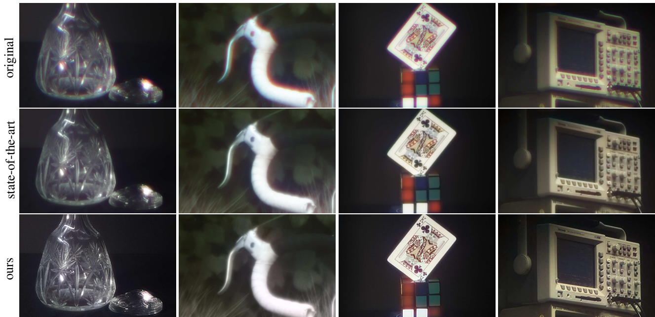
Figure 10: Restored images captured by a diffractive lens, suffering from severe chromatic aberration, with state-of-the-art reconstruction [6]. Zoom in for details.
