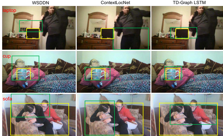
Figure 7. Qualitative comparisons with two state-of-the-arts on video object detection. The green boxes indicate detection results and yellow ones are the ground truth.
